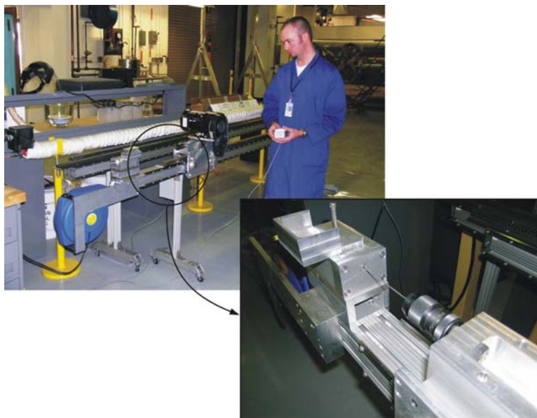
Figure 5. HTTL fixturing for fabricating drawn HTIR-TCs.
